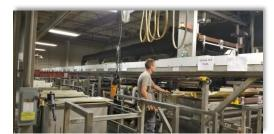
**Sulfuric Acid Anodization** (MIL-A-8625 Type III)
