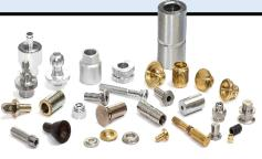
AO Precision's CNC equipment can turn parts as small as .375" ± .0005" in diameter and can mill parts as small as .250" x .250" ± .0005"
